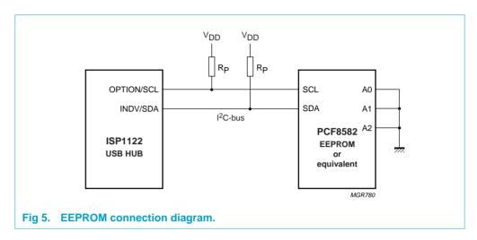
The slave address which ISP1122 uses to access the EEPROM is 1010000B. Page mode addressing is not supported, so pins A0, A1 and A2 of the EEPROM must be connected to GND (logic 0).
